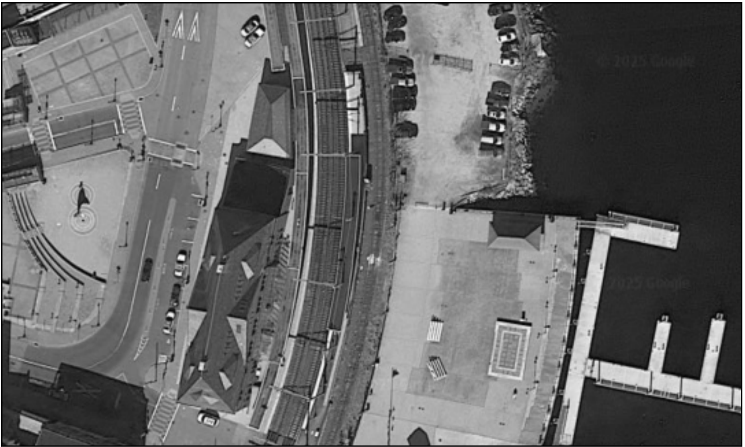
This satellite view of the New London, Conn. station shows the two passenger tracks (left and center) and the freight bypass (right)
